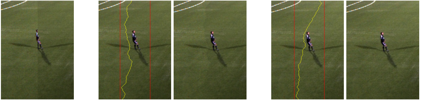
(a) The original stitch pipeline in [8]: a fixed cut stitch with a straight vertical seam, i.e., showing a player getting distorted in the seam.
