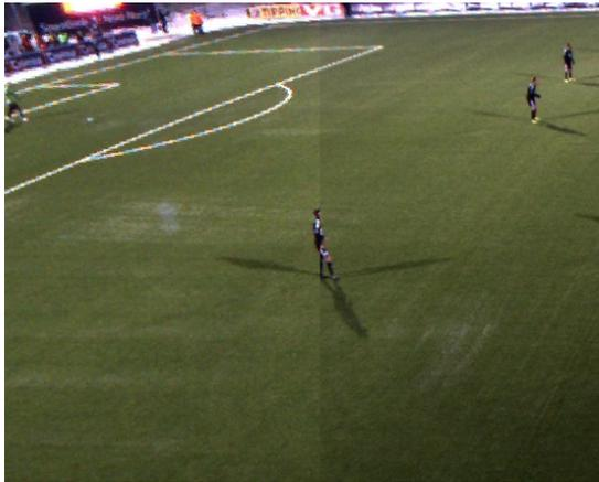
(a) Fixed cut stitch with a straight vertical seam, i.e., showing a player getting distorted in the seam.
