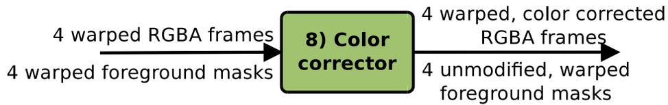
Figure 3.13: The Color Correction module
