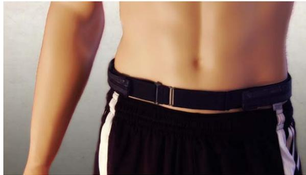
(a) Sensor belt used in the ZXY-system
