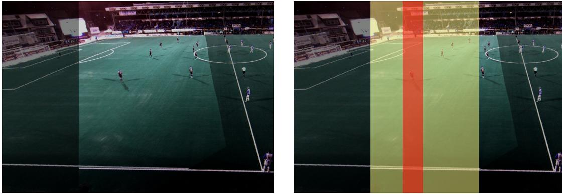
(a) Overlapping section between two warped frames. (b) Yellow shows suitable area for search. Red shows typical seam search area 100px wide.
