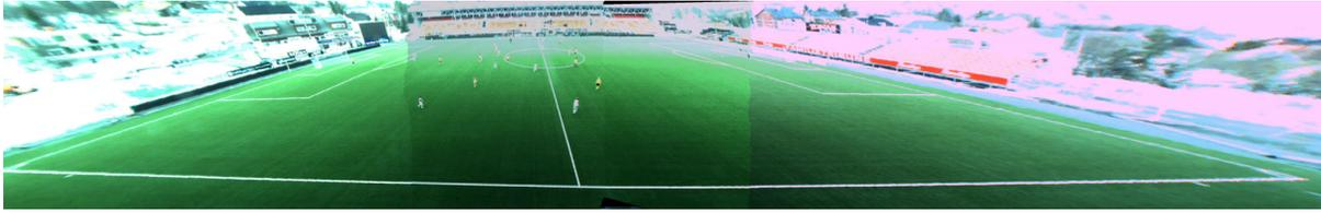
Figure 4.7: Dynamic stitcher output, here shown in full using an earlier color corrector version and experimental white balance correction in our camera driver.
